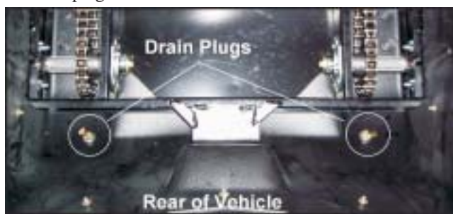
Figure 5-1. Location of rear drain plugs
