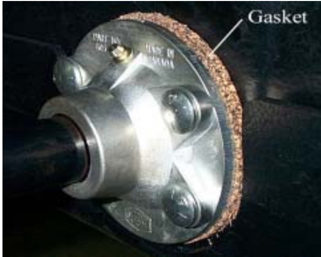
Figure 7-18. Bearing Flange and Cork Gasket
