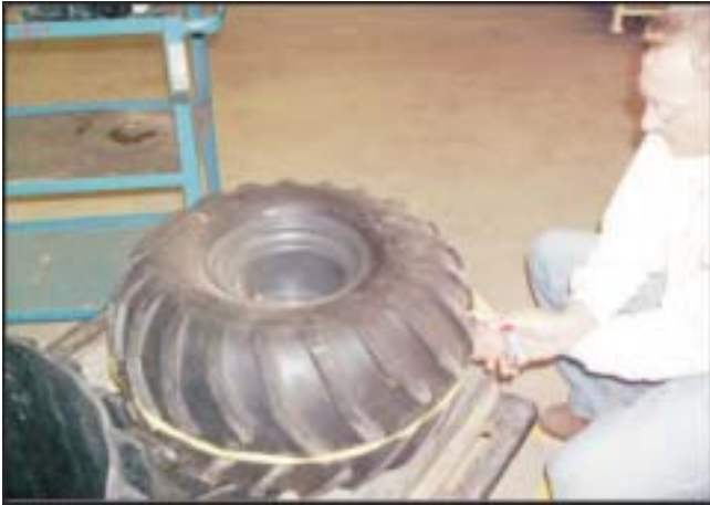
Figure 11-7. Measuring the tire.
