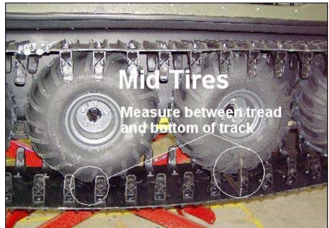
Figure 11-11. Measuring the gap of the mid tires - Avenger.
