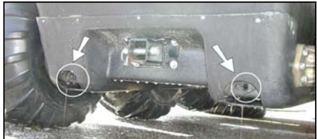
Figure 5-1. Location of rear drain plugs.
