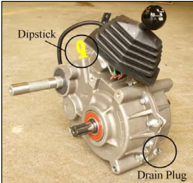
Figure 6-4a. 34-100 Transmission showing dipstick and drain plug locations
