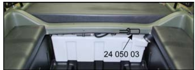
Figure 6-6. HDi and Avenger EFI fuel filter location.
