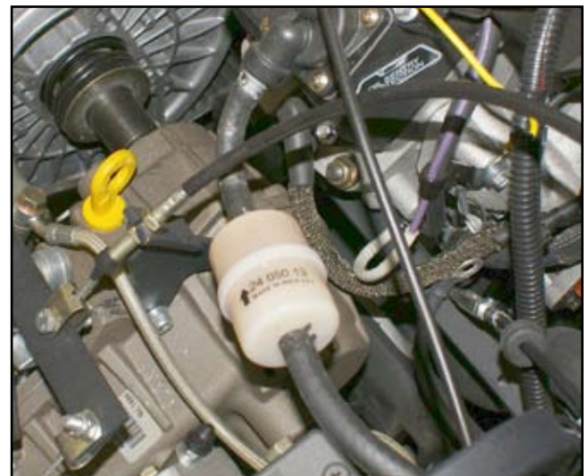
Figure 6-6a. Avenger 700 fuel filter location.
