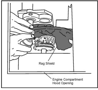
Figure 6-8. Lubricating the idler chain.
