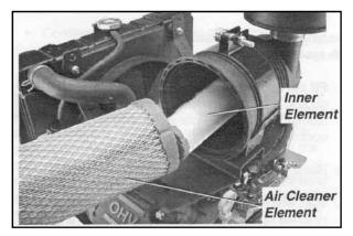
Figure 6-5a. Air Cleaner Element and Inner Element.
