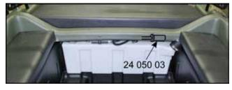
Figure 6-6. HDi and Avenger EFI fuel filter location.
