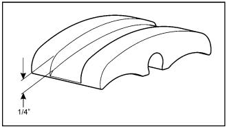
Figure 7-9. Wear groove on the slider block.
