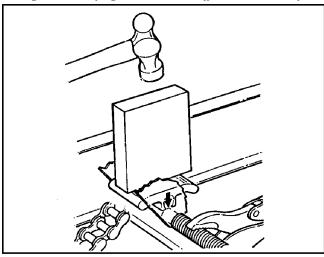
Figure 7-11. Hammering Slider Block into place.
