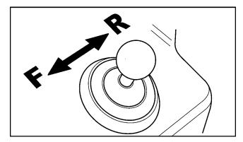
Fig 3-6. HDi gear shift travel and gear positions.
