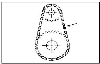
Figure 7-14. Position of idler chain link for removal.
