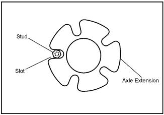
Figure 11-4. Check Stud Position in Axle Extension.
