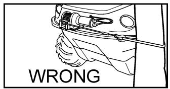
Figure 11-21. Incorrect positioning for continuous pulls.
