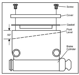
Figure 7-17. Hydraulic brake cylinder and fluid level
