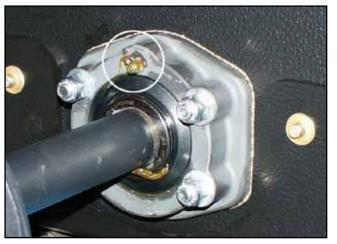
Figure 6-10. Outer bearing flange.
