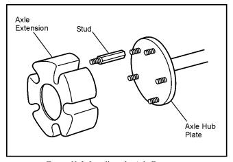
Figure 11-3. Installing the Axle Extensions.
