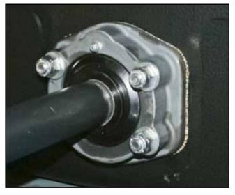
Figure 7-15. Bearing Flange and Cork Gasket
