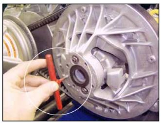
Figure 7-2a. Drive belt removal.
