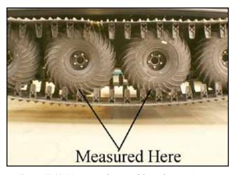
Figure 11-11. Measuring the gap of the mid tires - Avenger.
