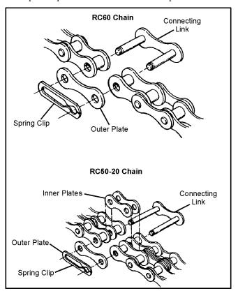
Figure 7-6. Chain connection link components.
