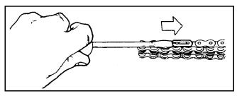
Figure 7-5. Removal of the spring clip.
