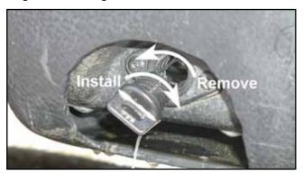
Figure 5-2. Removing and Installing the drain plug.
