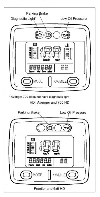
Figure 2-1. LCD Instrument Cluster.
