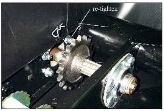
Figure 7-16. Re-tightening bolts.
