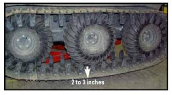
Figure 11-13. Measuring the gap of the mid tire - Frontier.
