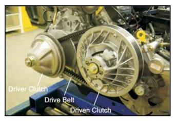
Figure 7-2. Location of drive clutches and drive belt.
