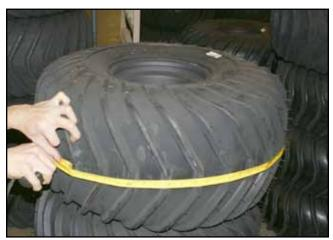
Figure 11-5. Measuring the tire.
