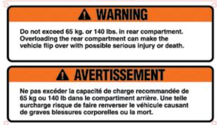
Figure 1-2 Rear Compartment Capacity Label - All 6x6 Models
