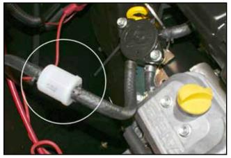
Figure 6-6b.Frontier fuel filter location.
