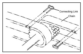
Figure 7-7. Installing the connecting link
