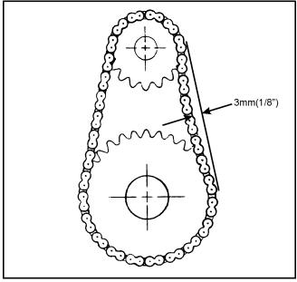
Figure 7-12. Measuring idler chain deflection
