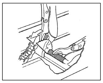
Figure 7-10. Prying the Slider Block off the Cam Assembly.
