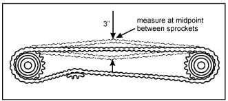
Figure 7-8. Chain slack required before the tensioner will progress to the next step.
