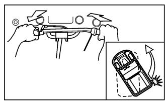
Figure 3-1. Making a left hand turn.
