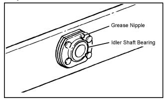
Figure 6-11. Inner axle flange grease nipple.
