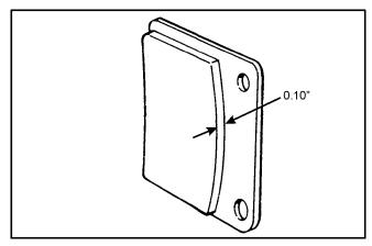
Figure 7-18. Brake pad wear, hydraulic brakes.
