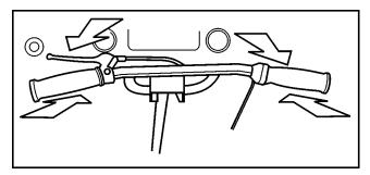
Figure 4-1. Position of moto-cross style steering bar in straight ahead operation.
