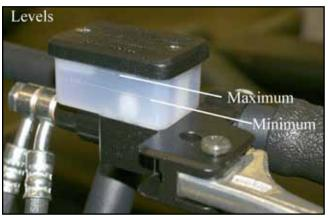
Figure 7-19a. Hydraulic handbrake levels
