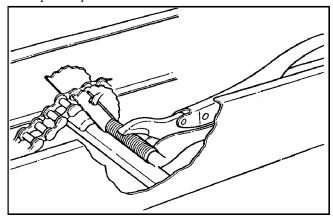
Figure 7-4. Securing tensioner cam
