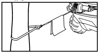
Figure 11-20. Using a cloth damper.
