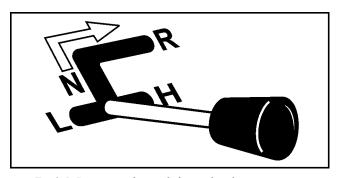
Fig 3-5. Direction of gear shift travel and gear positions.
