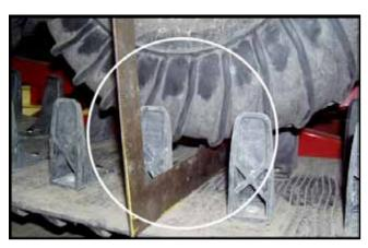
Figure 11-14. Measuring the gap of the mid tires - Frontier.
