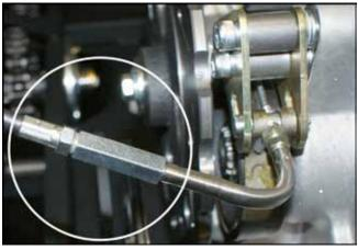
Figure 7-19c. Adjusting the parking brake.
