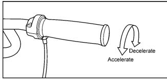
Figure 3-2. Operation of the throttle twist grip
