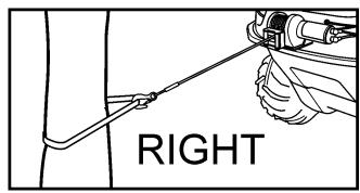
Figure 11-22. Correct positioning for continuous pulls.
