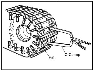
Figure 11-10. Securing with C-clamps.
