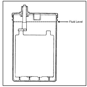
Figure 7-1. Battery fluid level
