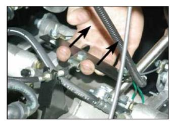
Figure 7-21. Equalizer Flat Bar.
