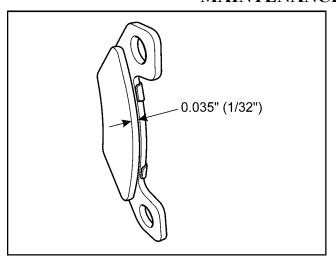
Figure 7-19b. Brake pad wear, HDi handbrake pads
