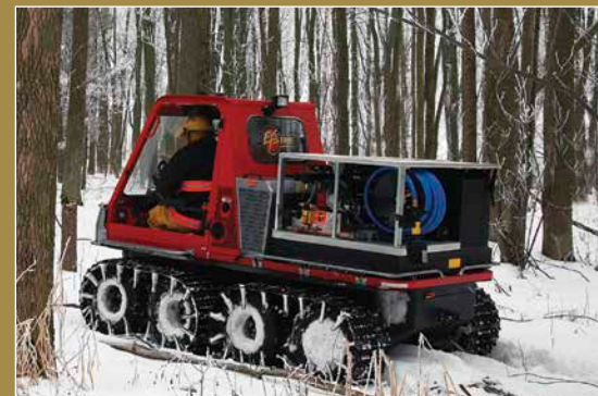
8x8 Centaur with customized equipment for emergency response
