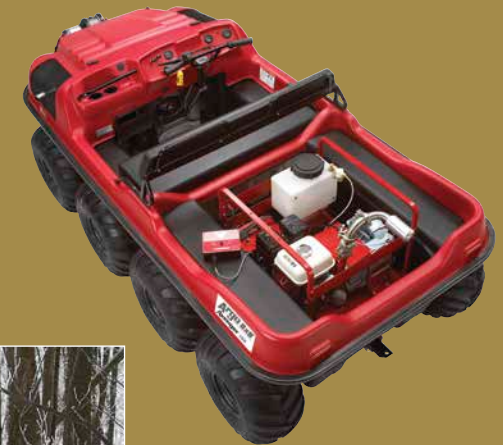
ARGO 8x8 750 HDi with spraying equipment for insect abatement
