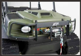
Halogen headlights, optional brushguard, 4,000 lb (1,814 kg) power winch (optional) and skid plate for lower body protection.
