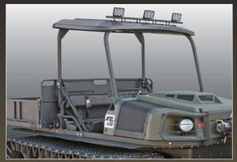
Optional, certified ROPS for two or four passengers is available with hard top for sun / rain protection and a light bar to add auxiliary lighting.
