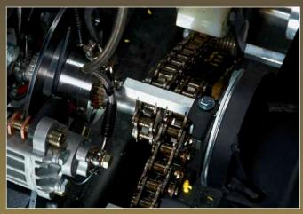
Optional automatic chain lubrication system featuring reduced maintenance requirements and longer chain life.
