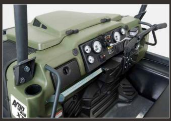
Multi-position steering system, instrumentation panel and convenience package (two cup holders, two storage compartments and two 12 volt outlets).
